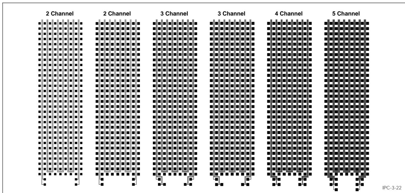
Figure 3-22 Conductor routing capability test pattern
