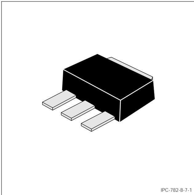
Figure 1 SOT 89 construction
