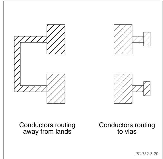
**Figure 3–20 Conductor routing**
