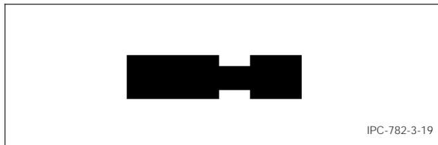
**Figure 3–19 Narrowed conductor**
