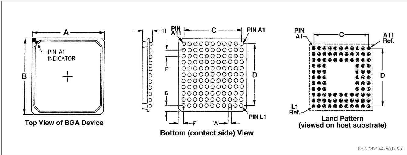
Figure 4-6 Device orientation and contact A1 position
