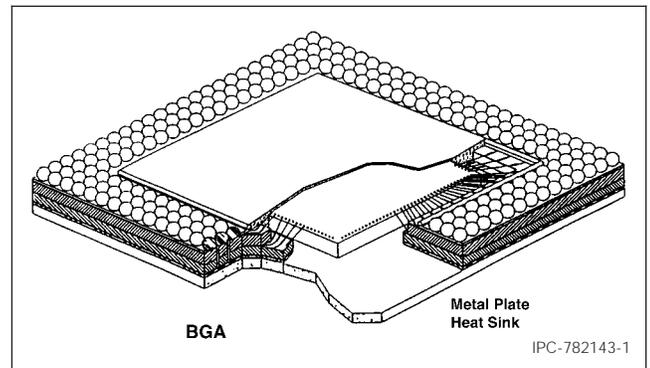
Figure 3-1 Ball Grid Array IC package example
