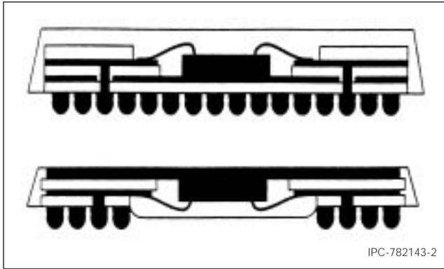
**Figure 3-2 Examples of plastic BGA package configurations**
