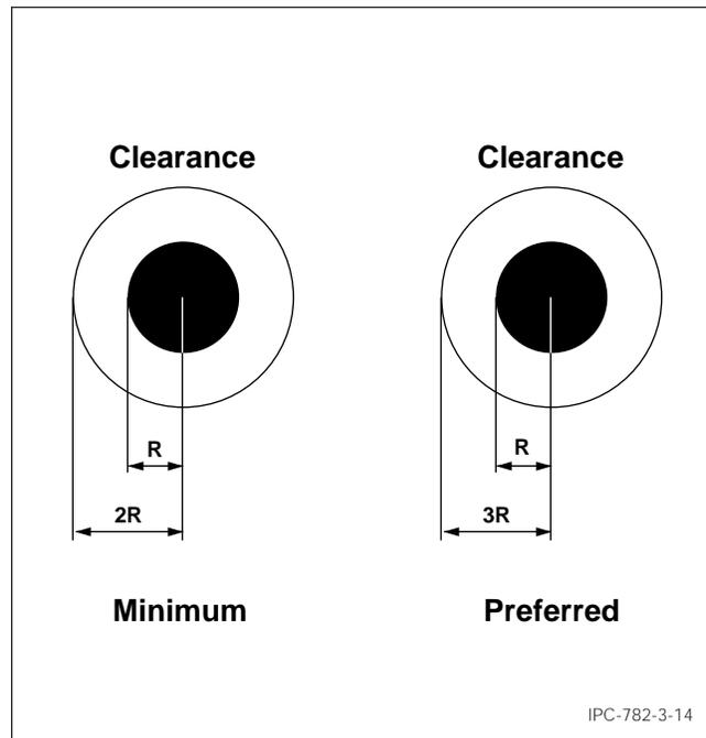
Figure 3-14 Fiducial clearance requirements
