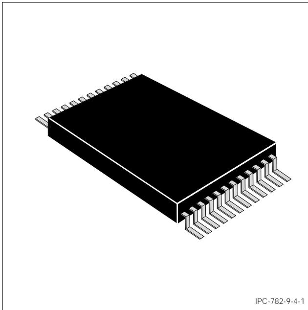
Figure 1 TSOP construction
