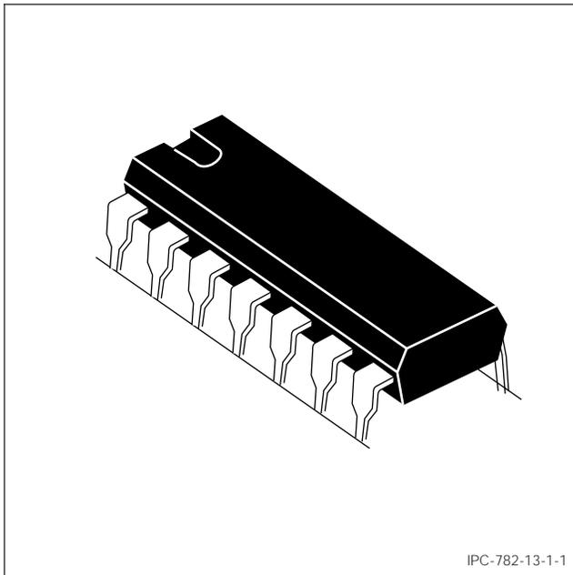
Figure 1 DIP construction
