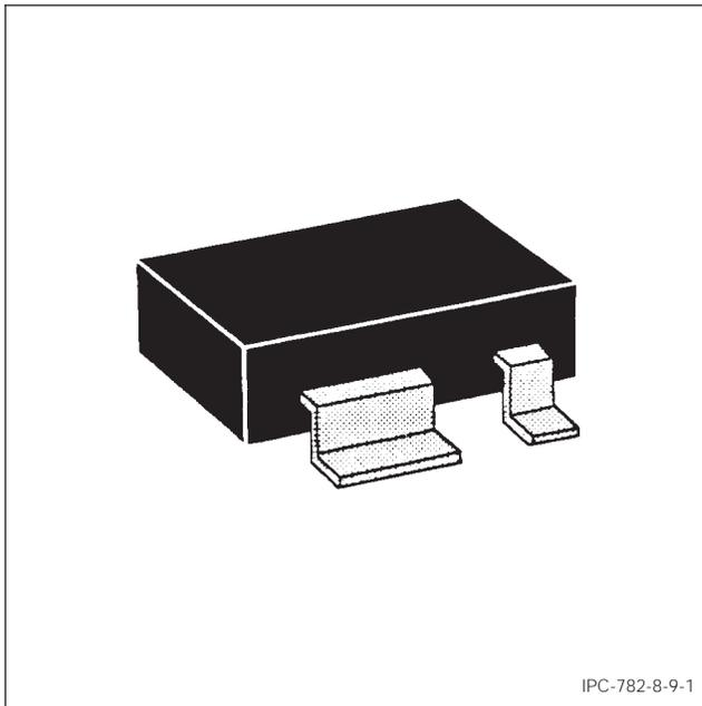
Figure 1 SOT 143 construction
