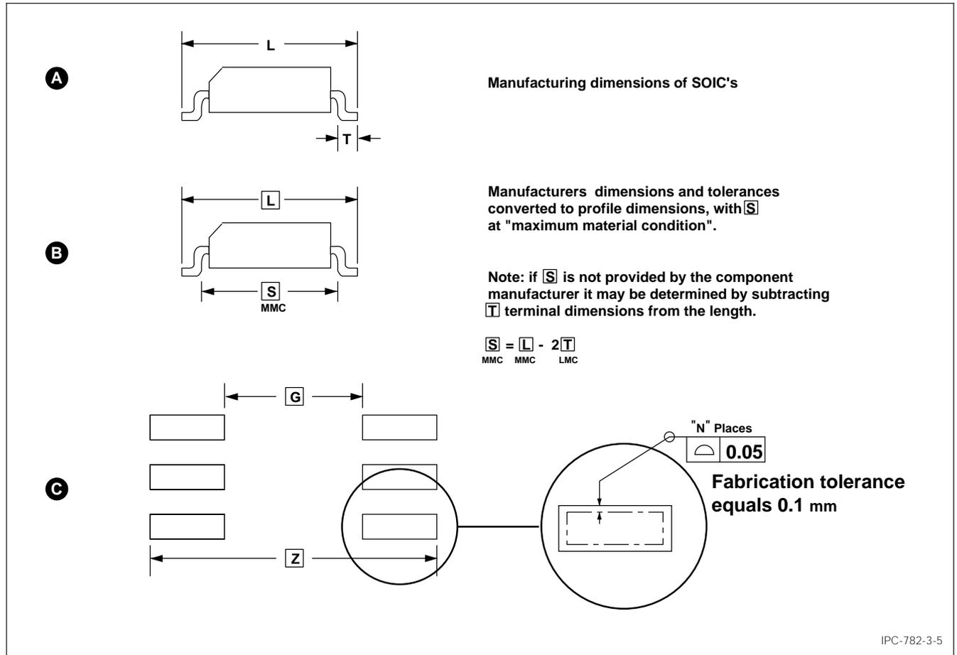
Figure 3-5 Profile dimensioning of a gullwing leaded SOIC
