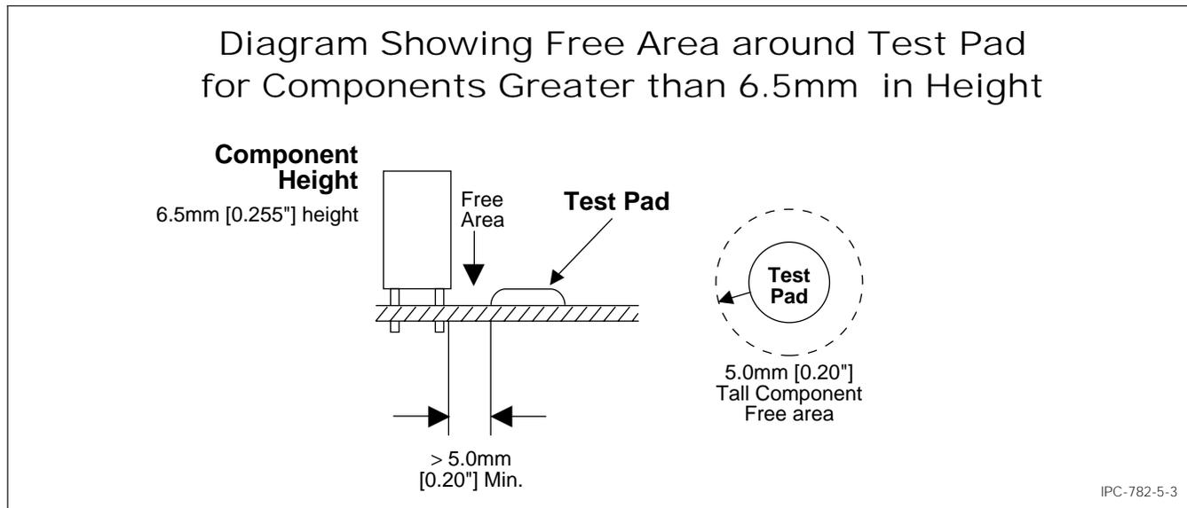
**Figure 5-3 Test probe feature distance from component**
