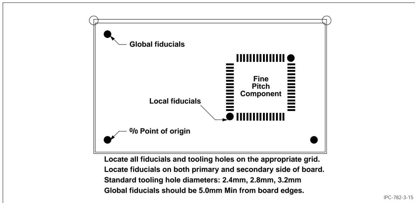
Figure 3–15 Fiducial locations on a printed circuit board
