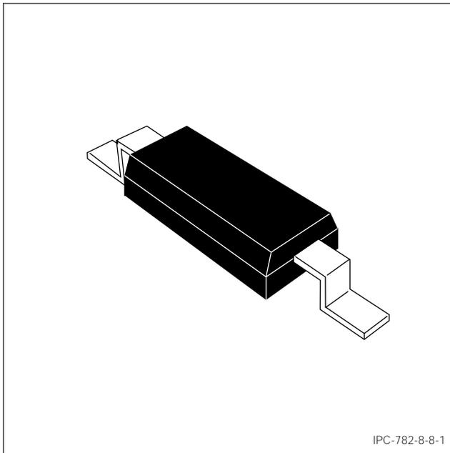
Figure 1 SOD 123 construction
