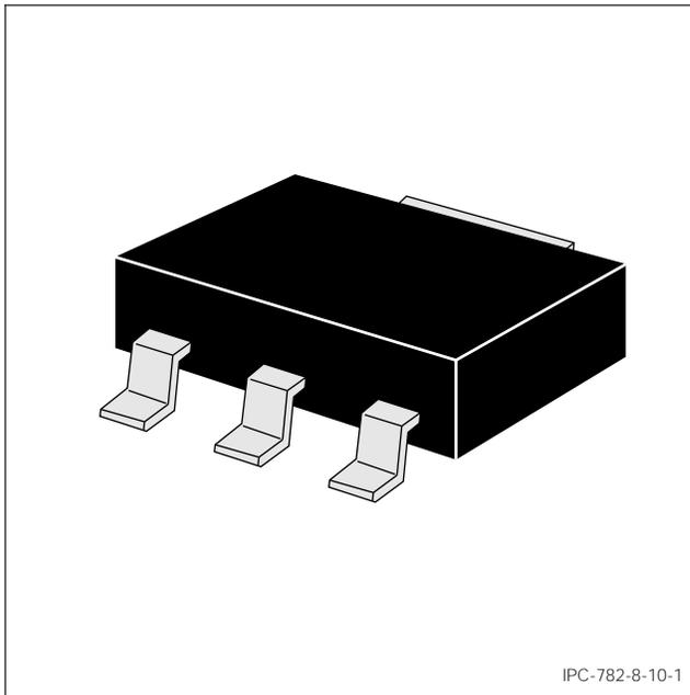
Figure 1 SOT 223 construction
