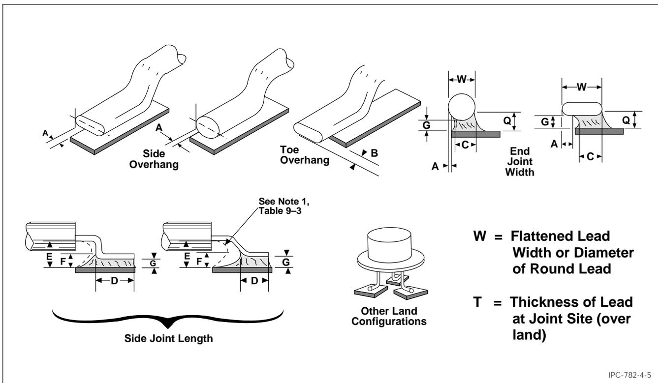
Figure 4-5 Round or flattened (coined) lead joint description
