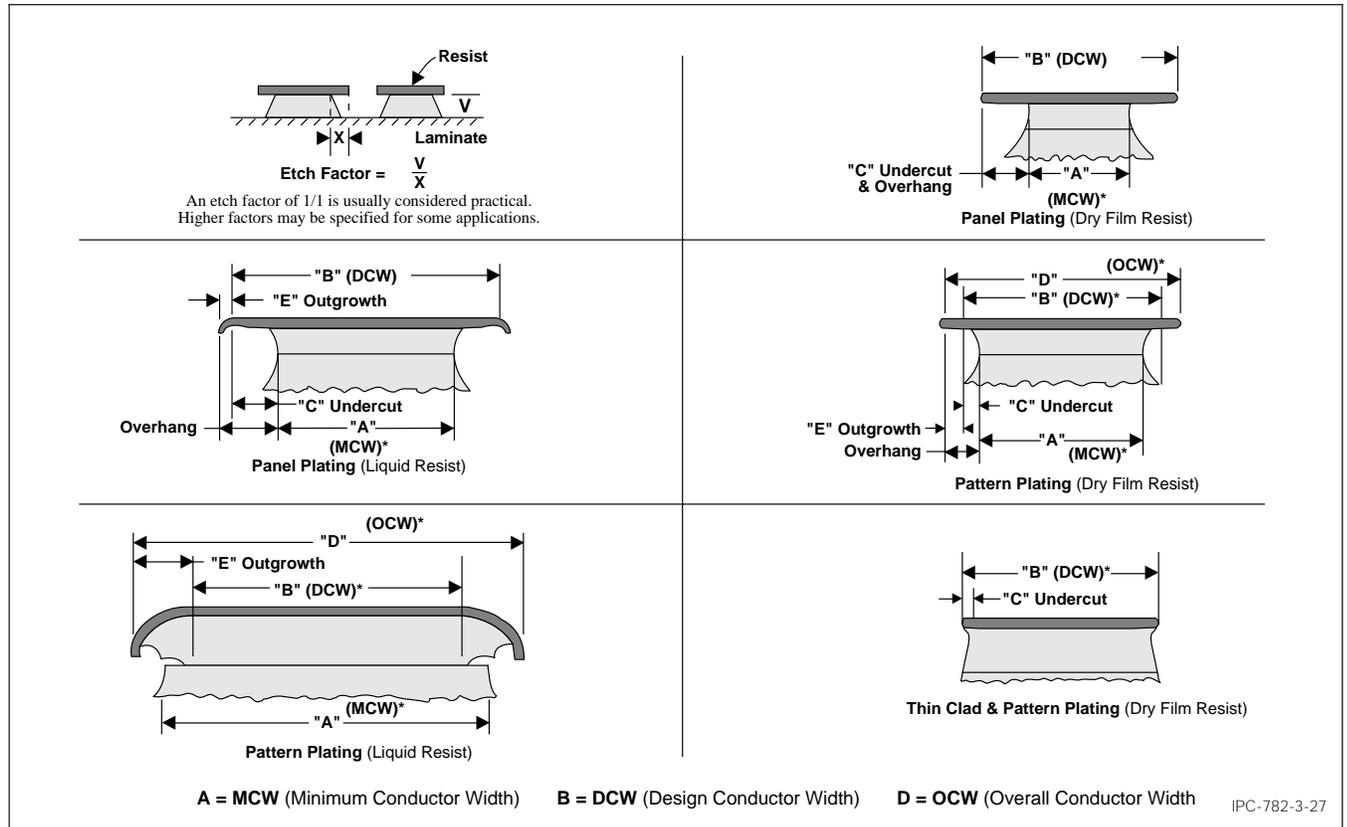
Figure 3-27 Conductor characteristics
