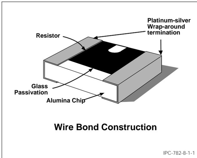
Figure 1 Chip resistor construction
