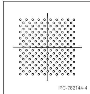
Figure 4-4 Staggered matrix
