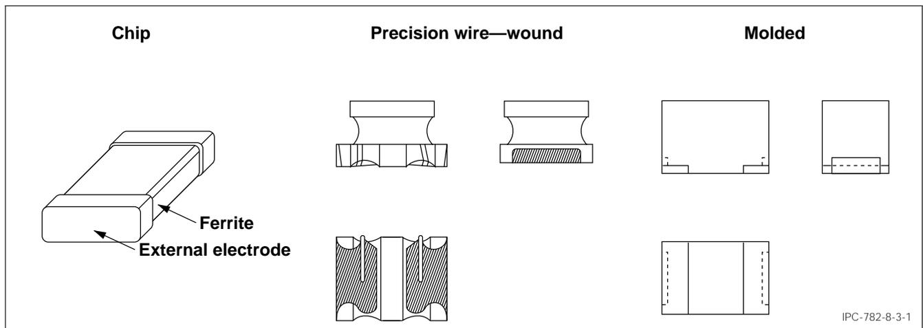
Figure 1 Inductor construction
