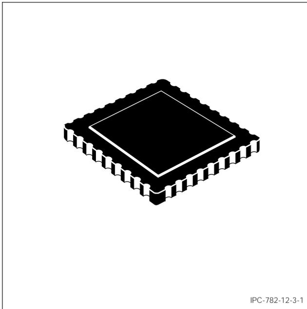
Figure 1 LCC Construction
