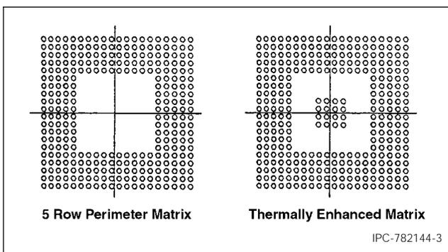
Figure 4-3 Perimeter and thermally enhanced matrices
