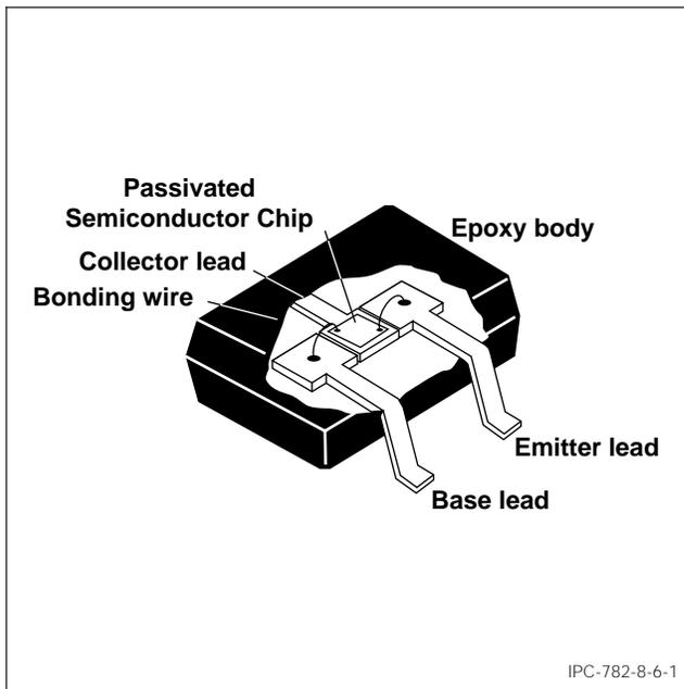
Figure 1 SOT 23 construction
