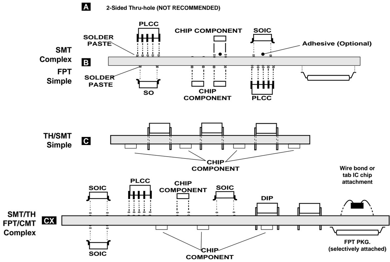
Figure 1-1 Electrical assembly types
