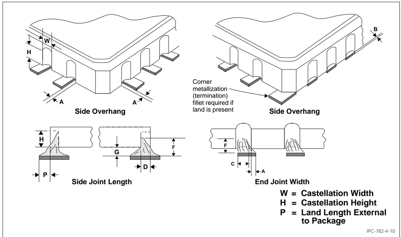
Figure 4-10 Leadless chip carriers with castellated terminations—joint description
